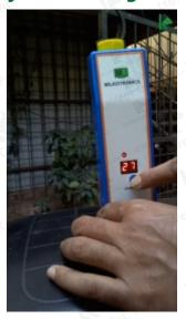
1.8 The temperature display indicates rise in the water temperature. The vibrator activates at 33°C. Water inside heats to 37°C in 3-4 minutes and stays constant. At 37°C, it beeps twice. Thus, DFSTS is now ready for thawing.
