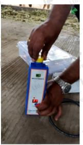
**3.4** After 30 seconds the DFSTS beeps 3 times and the red LED on the front of the DFSTS turns on. Thus the thawing is known to be complete.
